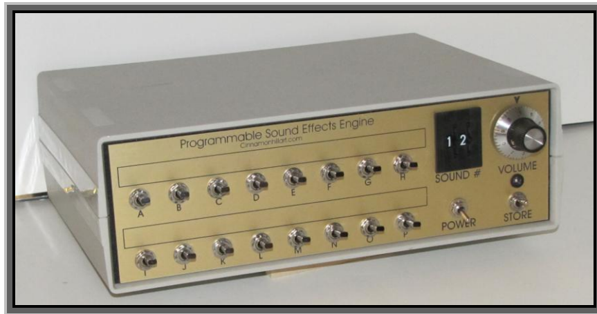
Photo #1: The complete Programmable Sound Effects Controller. The “wall-wart” power supply is not shown.
