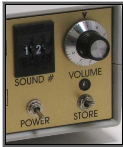
Photo #3: The programming section of the Programmable Sound Effects Controller
